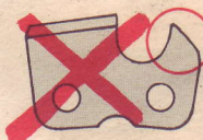
WRONG: NOT ENOUGH STRAIGHT SECTION LEFT TO ACT AS DEPTH GAUGE.
